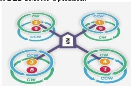
FIGURE 4.1 DYNAMICS OF COAXIAL QUADCOPTER
